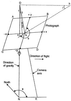
In above figure, oi is the bisector and 'i' is the isocentre. The angle of tilt lies in the principal plane, and hence the isocentre (i) lies on the principal line at a distance of f  $tan \frac{t}{2}$  from the principal point, where t = tilt and f = principal distance. On a vertical photograph, the isocentre and the photo- nadir point coincide with the principal point.
